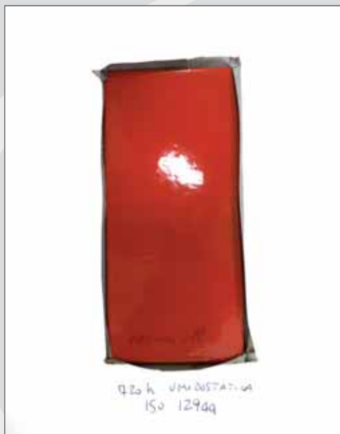
Condensation in water Condensa in acqua
